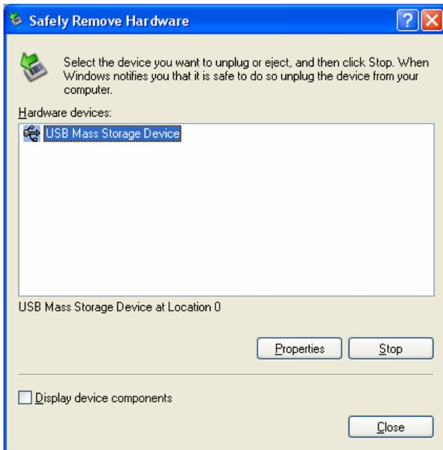
A message will appear indicating that the portable storage device can now be securely removed. If a message saying “The ‘...’ device cannot be stopped right now” appears, you have to close your Windows Explorer or any other application that is still accessing the data on the USB Drive.
